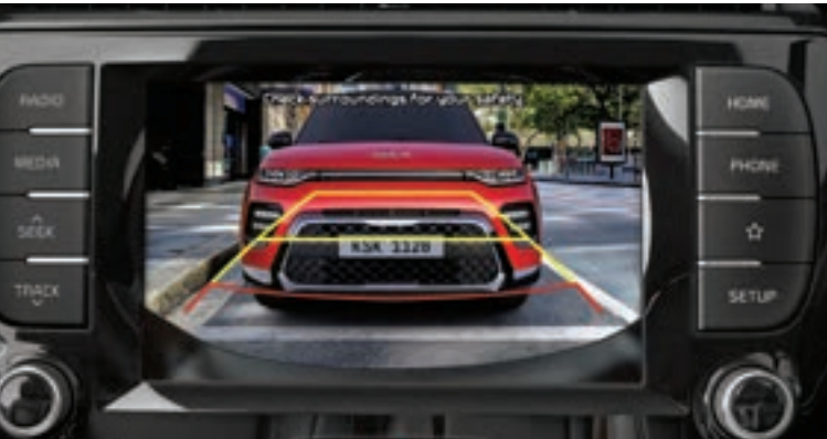
Rear View Monitor (RVM) : Rear top view Dynamic parking guidance adjusts its guide lines as you turn in reverse for precise parking, and now features a top view option on the center screen.
