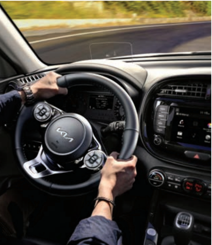
Ride & handling An electric motor on the steering column results in more responsive steering, while numerous chassis and body upgrades make the ride even smoother.
