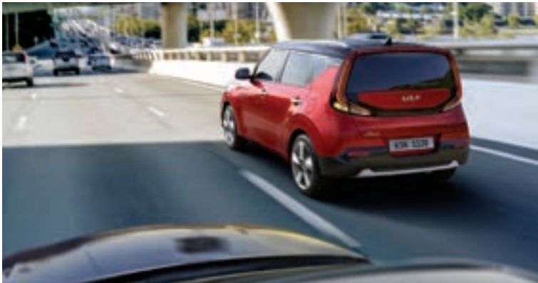
Blind-Spot Collision Warning (BCW) Using radar technology, BCW monitors your sides and rear and warns you if it detects a vehicle approaching into your blind spot from behind or adjacent lanes of travel. The system issues visual alerts on the side mirror and an audible alert.
