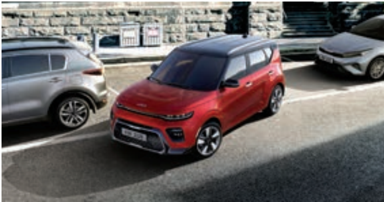
Parking Distance Warning-Forward (PDW-F) To help you park safely and confidently, PDW-F uses ultrasonic sensors mounted on the front bumpers and uses visual alerts on the side mirrors as well as audible alerts to warn you of any vehicles or obstacles ahead that may be getting too close.
