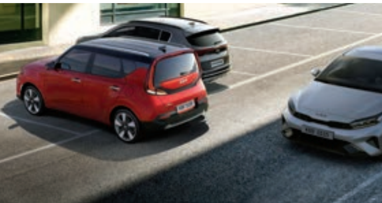
Rear Cross-Traffic Collision Warning (RCCW) As you reverse out into a traffic lane, RCCW (manual transmission-equipped models only) scans the area using radar, and warns you with an audible alert signal if it senses a vehicle approaching. On automatic transmission-equipped models, Rear Cross-Traffic Collision-Avoidance Assist (RCCA) also uses ESC to brake, help avoid a collision or reduce damage.
