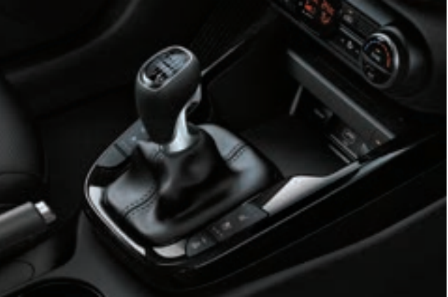
6-speed manual transmission Enjoy dynamic shifting, quicker reverse-gear engagement, and better fuel efficiency with the durable 6-speed manual transmission.
