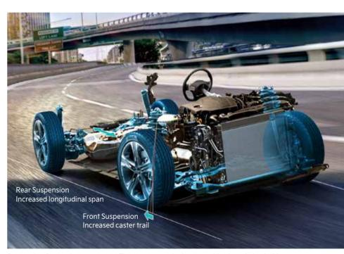
Suspension System Improvements The rear suspension's arm position is optimized with an increased longitudinal span. At the front, the caster trail is increased for better wheel recovery after cornering. As a result, the K5 is more responsive and agile, as well as more fun to drive.
