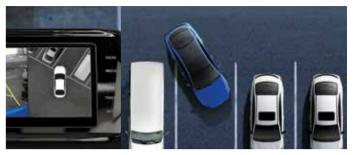
Surround View Monitor (SVM) When operating in confined spaces, multiple cameras provide you with a zoomable, 360° overhead view of the vehicle's surroundings, so you can maneuver with confidence and without having to get out of the vehicle.
