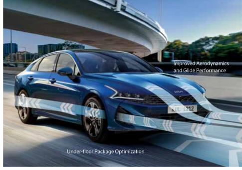
Multi-faceted Aerodynamics The K5 manages airflow in new and efficient ways. Front air intakes cool the brakes while the air that cools the engine space flows rearward freely under the cabin.
