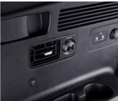
3rd row air conditioning system
