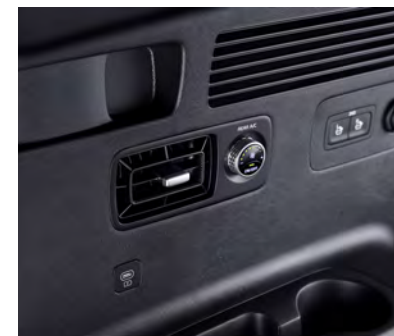
3rd row air conditioning system
